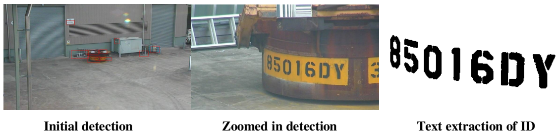
Figure 7. Identifying a crucible label in the environment without initial knowledge of its location.
