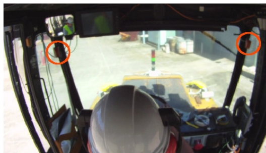
Figure 6. Lights mounted inside the cabin (orange circles). During manual operation, these lights alert the driver of a potential collision route between the vehicle and a nearby pedestrian.
