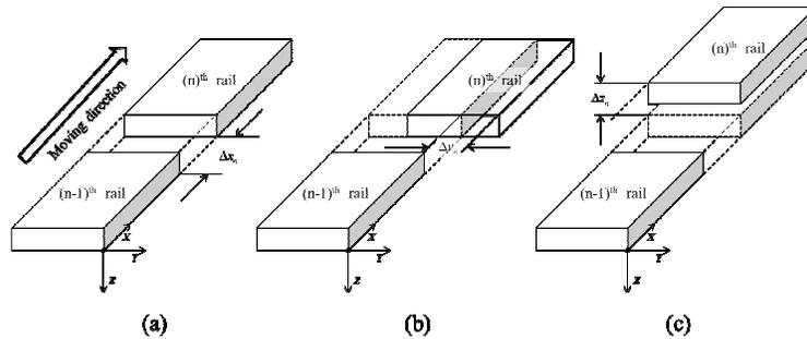
Figure 4 – Definition of error related with rail-joint: (a) X-axis, (b) Y-axis, (c) Z-axis direction
