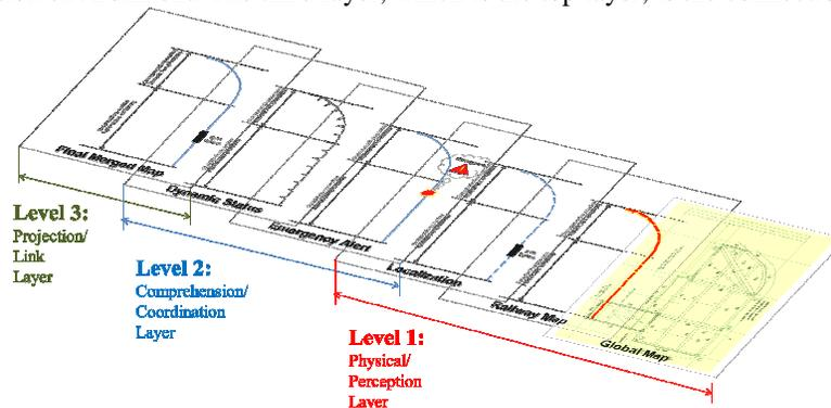
Figure 2 – Layered architecture of HSM control
