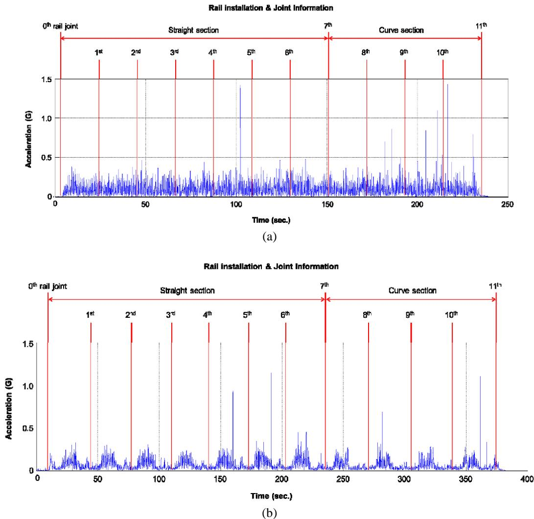
Figure 8 – Experimental Result for acceleration of the HSM: (a) without motion control algorithm, (b) with motion control algorithm
