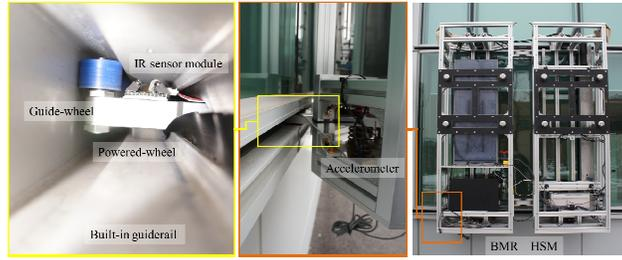
Figure 3 – Configuration of sensor integrated HSM
