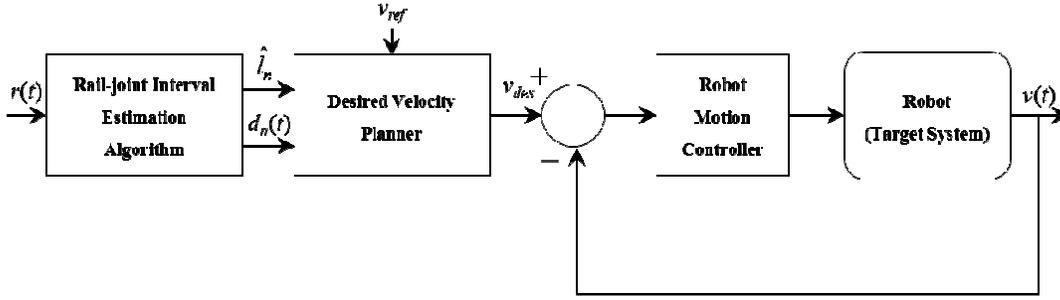
Figure 7 – Block diagram for motion control of HSM
