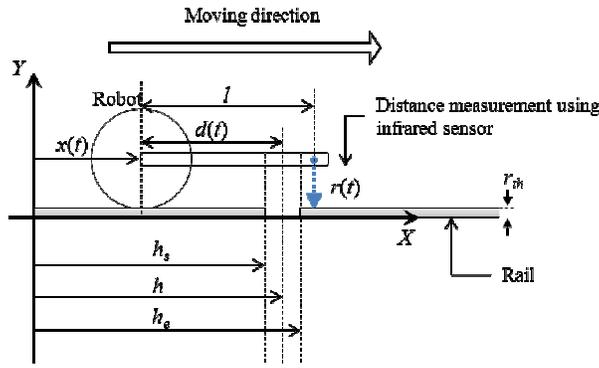
Figure 5 – Definition of error related with rail-joint: (a) X-axis, (b) Y-axis, (c) Z-axis direction
