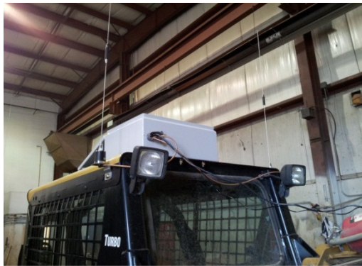
Figure 3: RFID Readers for JV Driver fabricators' site
