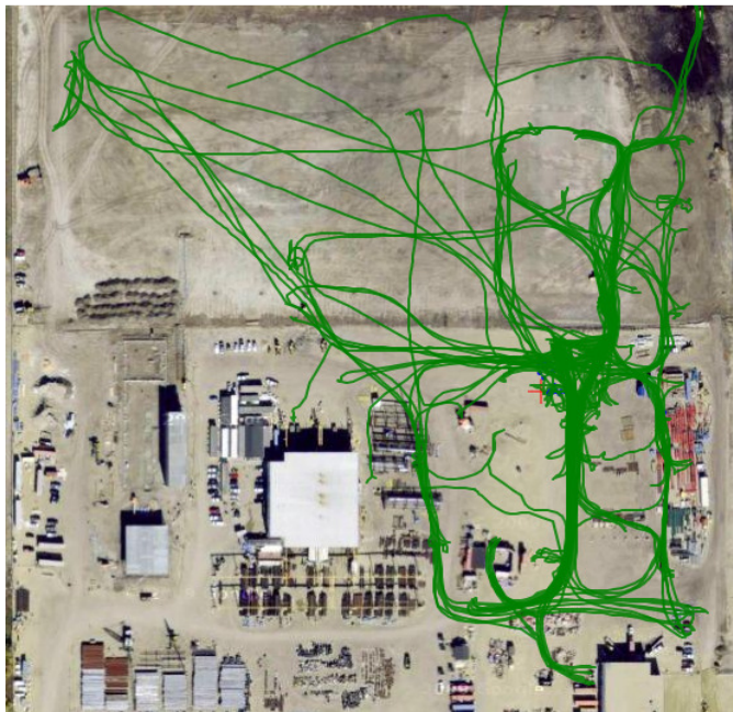
Figure 4: RFID Reader-Enabled Vehicles' (ROVER) movement tracks in JV Driver Module Yard
