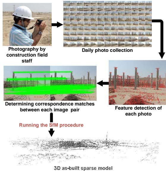
Figure 2. Process of collecting as-built data resulting in the reconstructed 3D as-built point cloud model
