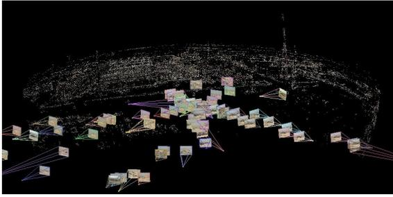
Figure 8. Sparse 3D model reconstructed from 99 images with camera frusta
