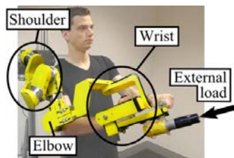
Figure 9. An 8-DOF scaled-down proof-of-concept prototype robot
