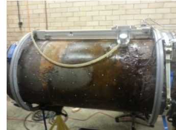
Figure 7. Section of a typical large water main exhumed from the ground and being inspected in a lab
