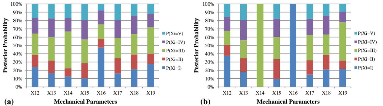
Fig. 6. Fault diagnosis under *Scenario D* in: (a) the first diagnosis cross  $P(T=IV)$ ; and (b) the second diagnosis cross  $P(T=IV|X_{14}=III, X_{16}=I)$ .
