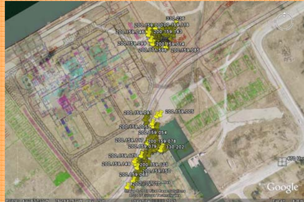
Pipe spool locations using automated materials tracking
