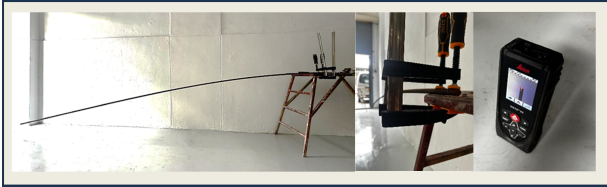
Figure 5. Rebar deflection experiment set up
