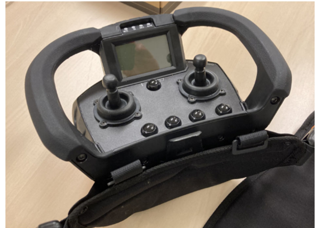
Figure 4. The wireless joystick control device used for remote control of the end-hose 2 .
