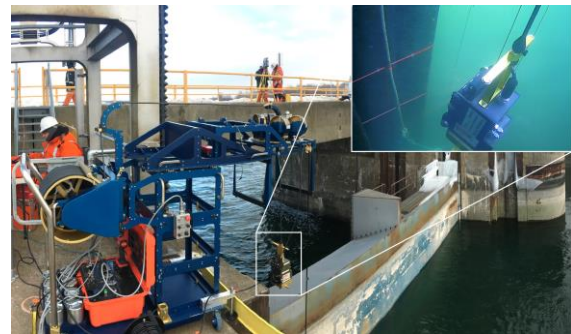
Figure 3. WireScan measurements on a spillway. Underwater scanning (top right). Modular multifunctional platform (left).
