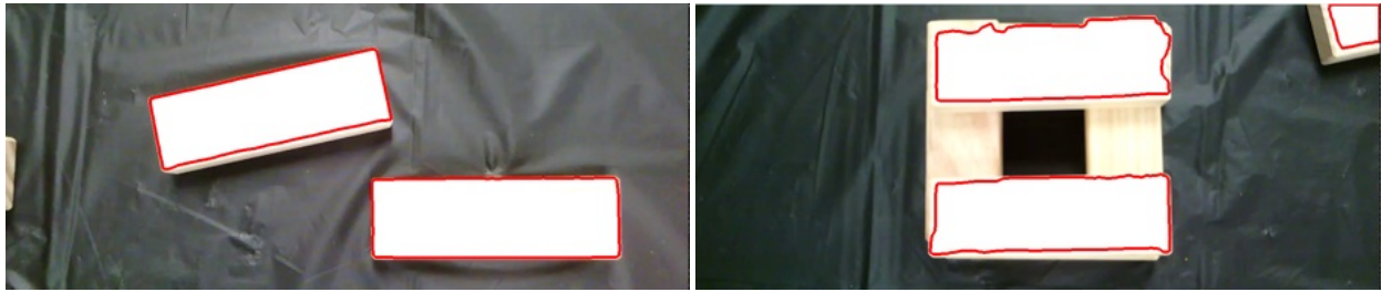
Figure 6. The robot camera's top view of two blocks and an assembled hollow tower. Red lines indicate detection results from the vision-based state estimation algorithm.
