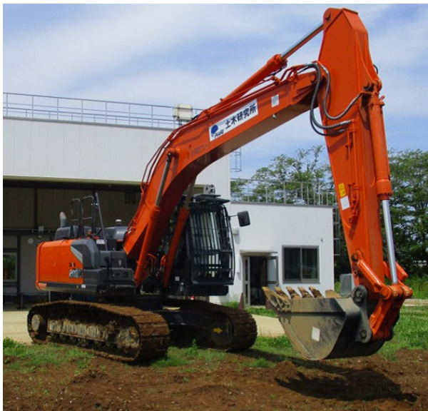
Figure 1. Developed excavator built-in velocity controller.
