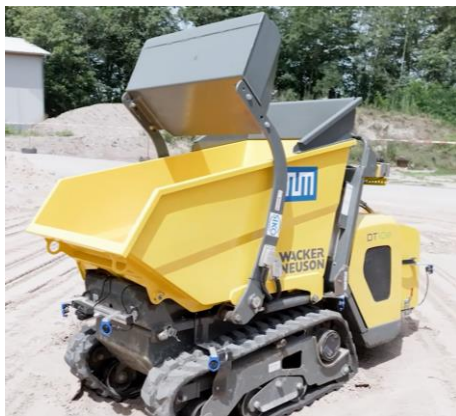
Figure 1. Autonomous dumper project, developed by TUM and Wacker Neuson
