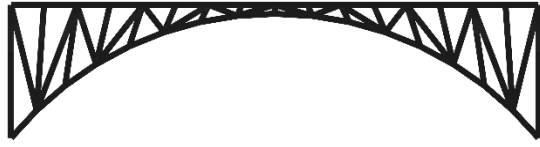
Figure 7. Optimized Truss Configuration for Unsymmetrical Loading
