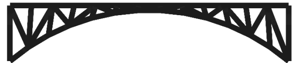
Figure 5. Optimized Truss Configuration for Symmetrical Loading
