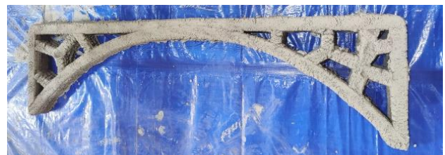
Figure 8. 3D printed Voronoi Lattice Beam
