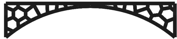
Figure 4. Optimized Voronoi Configuration for Symmetrical Loading
