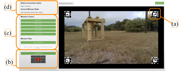
Figure 7. (a) Apriltag rendered in the corner of the Workspace area of the application. (b) Teleoperation interface for manual UGV operation. (c) Mission control buttons and file viewer. (d) Mission and connection state.
