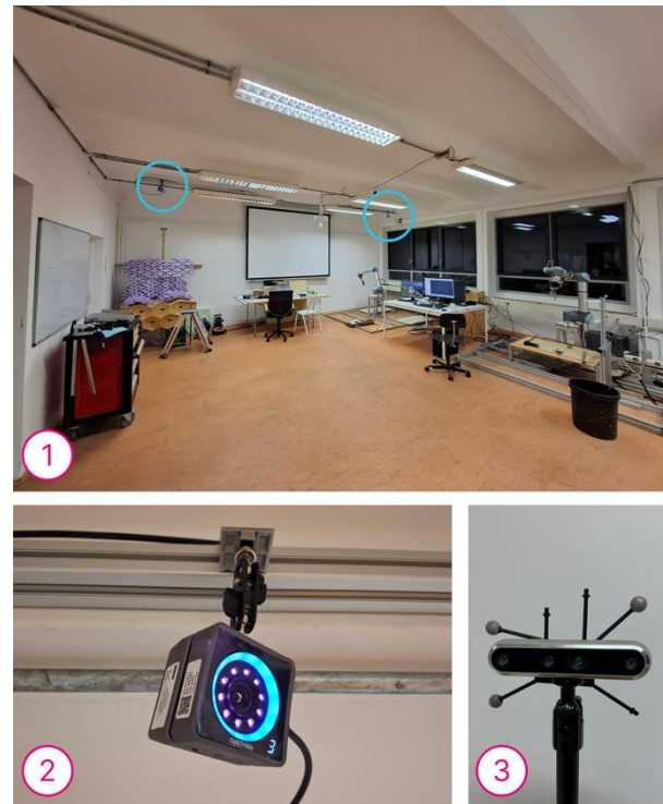
Figure 2. 1) Hardware setup in the case-studies lab environment (7x10m) consisting of 2) four OptiTrack Prime X 13 cameras (ground truth) and 3) a depth camera for localization (e.g. RealSense D455)
