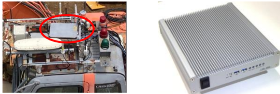
Figure 4. Ultra-low latency 4ch HD video encoder
