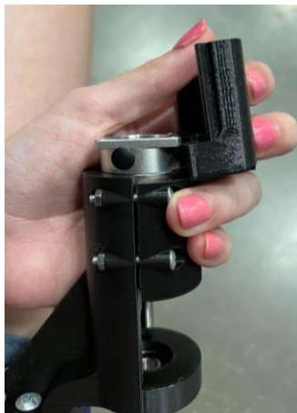
Figure 19: Motor Mount Too Thick
