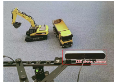
Figure 7. ZED camera fixed in a holder to capture stereo images of working construction machines.
