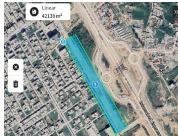
Figure 2. UAV flight planning for photogrammetry-based monitoring
