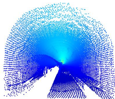
Figure 4. The view of the tunnel's interior is represented in the point cloud.
