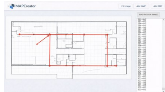
Figure 6. Routable path generation in Map Creator using the 2D floor plan.
