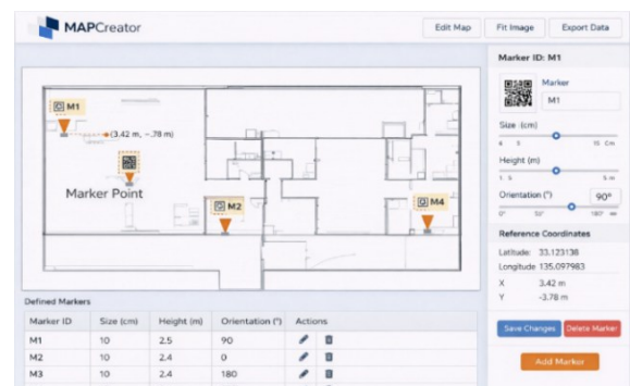
Figure 5. Marker point configuration and automatic generation of reference coordinates in Map Creator.
