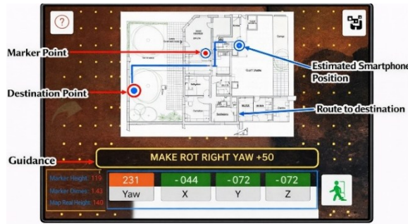
Figure 10. Smartphone screen showing the interface for indoor navigation
