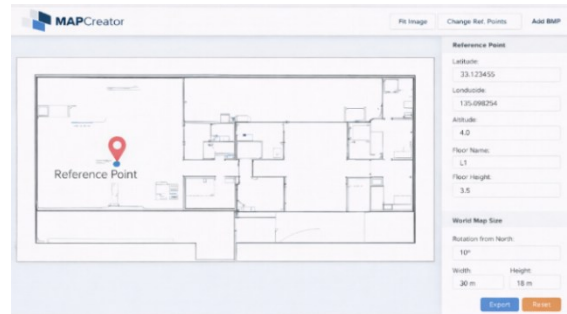
Figure 4. Map Creator screen with Floor Plan and associated geographic information.
