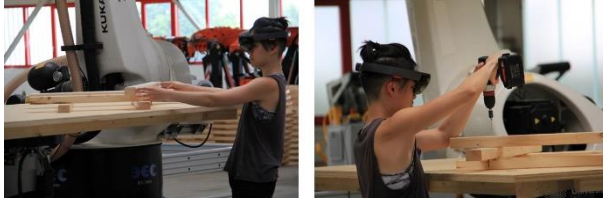
Figure 9. Same tasks executed with a different skill set by a Hololens-equipped human (slat fixation by screwing)
