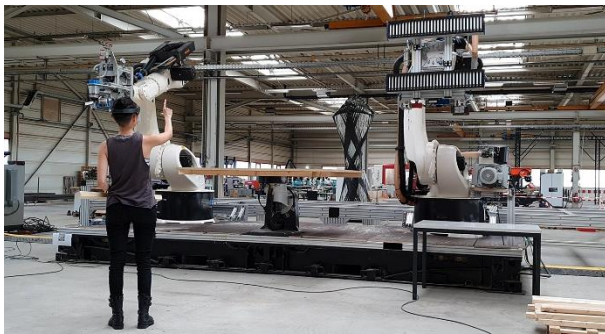
Figure 2. Human wearing an HMD controls the robotic fabrication setup
