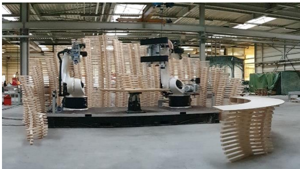
Figure 7. Trade show stand surrounding the robotic fabrication platform which fabricated it
