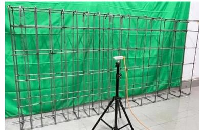
Figure 5. The double-layer bidirectional rebar cage
