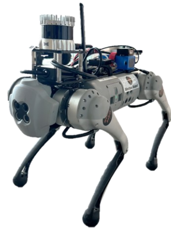
Figure 1. Quadruped robot equipped with 3D LiDAR sensor for automated 3D scanning
