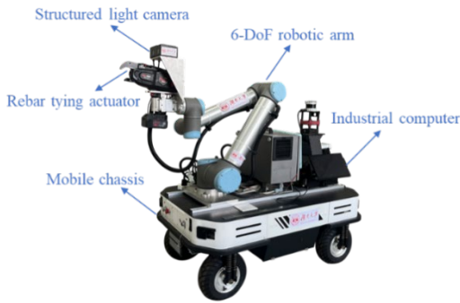
Figure 6. Rebar tying robot developed by our research group
