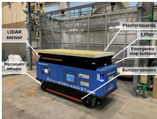
Figure 3. Assist robot for ceiling construction robot.
