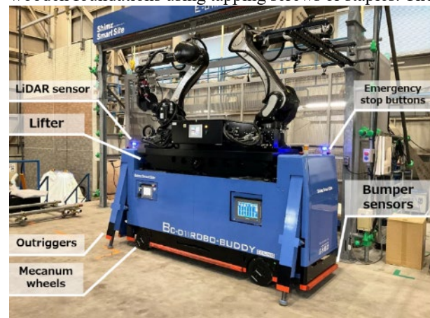
Figure 1. Ceiling construction robot.
