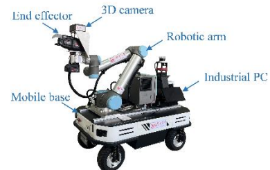
Figure 4. Rebar tying robot developed by our research team.
