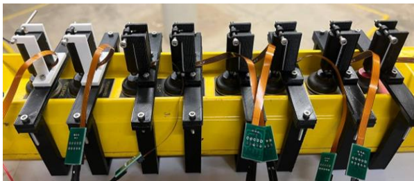
Figure 6. Crane remote control with mounts and actuators.
