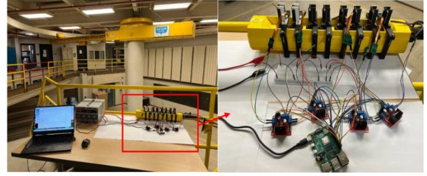
Figure 7. System setup for remote access crane.
