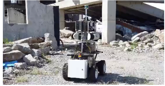
Figure 5. A mobile robot deployed to collect laser scans at the Guardian Centers disaster training facility.
