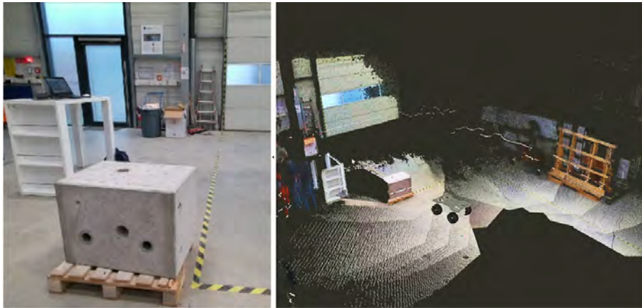
Figure 6. The visual feedback visualized to the user in the control PC (Left: 2D camera views in 640 x 576, Right: 3D map generated with the captured point clouds)
