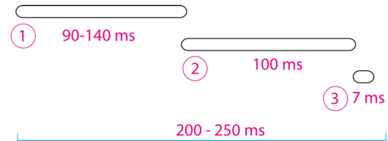
Figure 6. Approximated processing time 1) Path calculation (Python API time measure); 2) MQTT transfer (Mqtt-explorer timestamp); 3) GH path creation (GH profiler).
