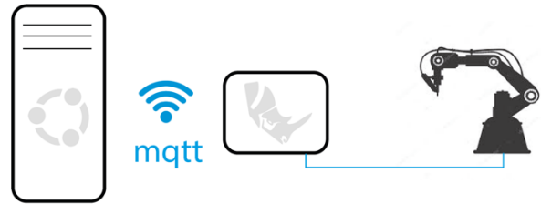
Figure 1. Scheme of the system setup: Left – Debian GPU workstation with cuRobo, connected to a GH user computer via an MQTT connection and to the robot via cable.
