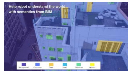
Figure 4. Aligning aerial photograph with BIM rendering to facilitate robot perception.
