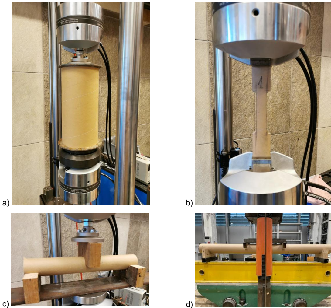
Fig. 1. The views of the samples during the tests: a) compression test, b) tension test, c) 3-point bending test, d) 4-point bending test on a full-scale sample.
