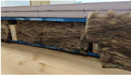
Figure 3. Testbed configuration for multiple layers of insulation
