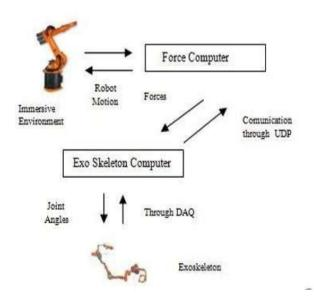
Figure 2. Communication between the KUKA manipulator and exoskeleton [10]
