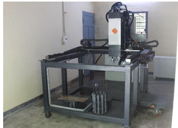
Figure 3 An early prototype of the design integrating 3D printing with robotic pick and place features
