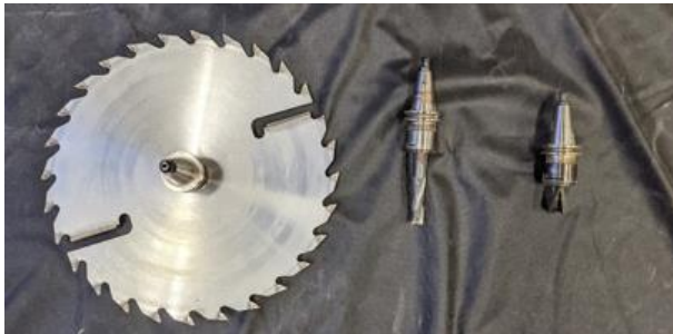
Figure 3 Tools used for raw wood processing. Chip saw (Left). Spiral bit (Center). Dovetail bit (Right).
