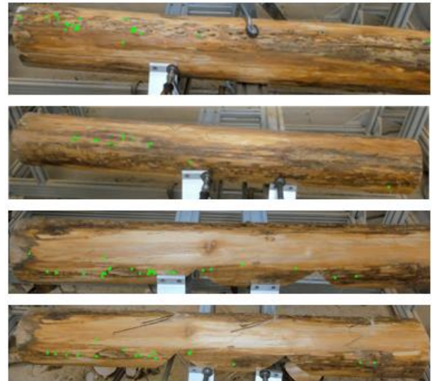
Figure11 Images taken from a camera installed in a processing machine and overlaid with the feature points used for position and orientation estimation. From top to bottom: before processing, once repositioned, twice, and three times repositioned.
