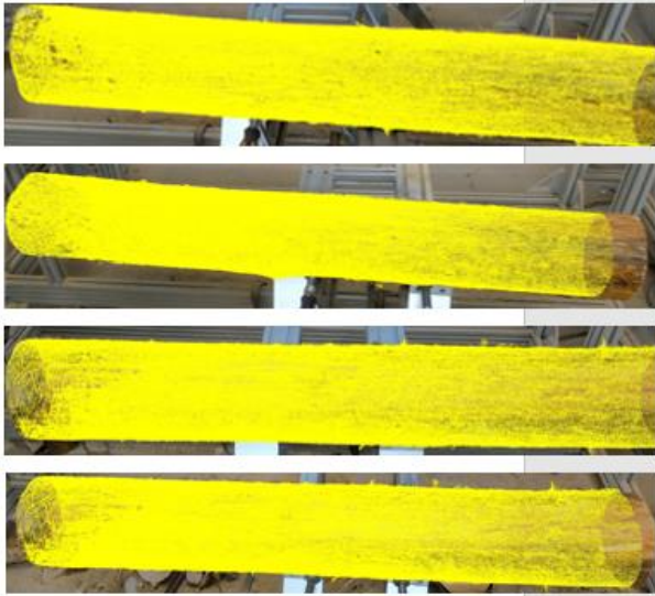
Figure 12 Images taken from a machine with shape data overlaid according to the estimated position and orientation. From top to bottom: before processing, once repositioned, twice, and three times repositioned
