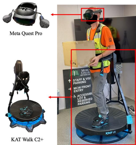
Figure 1. A participant performing material handling tasks in a virtual construction environment using a VR headset and omni-directional treadmill.
