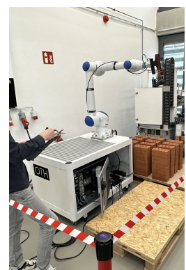
(b) Realization of simulated and optimized brick laying process integrating the Yaskawa HC10 at the Building Lab of OTH.
