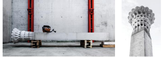
Figure 2. FDM formwork process map and results (credit: digital building technologies, ETH Zurich)
