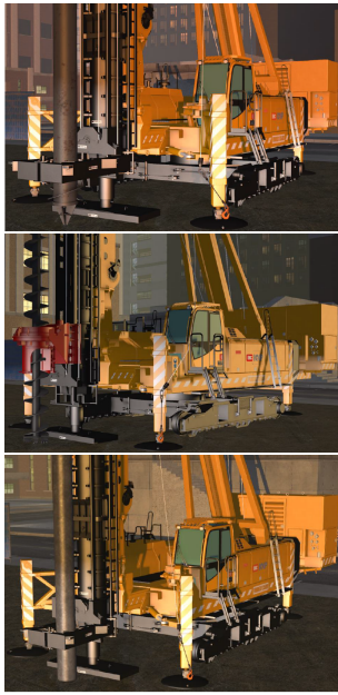
Figure 1. Displacement pile (top), continuous flight auger (middle) and hydrohammer (bottom) on a drill rig
