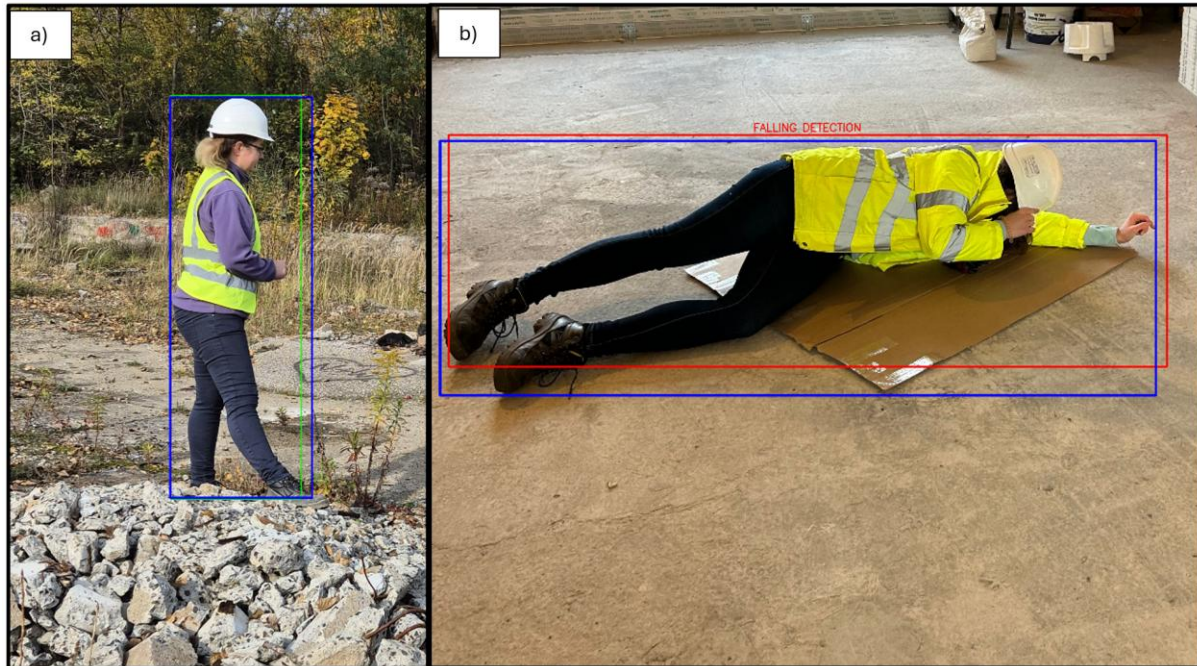
Fig. 3. Output frames from the image-analysis process using the developed algorithm: (a) no human fall detected; (b) human fall detected.
