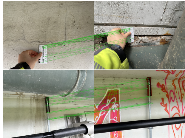
Figure 8. False positives for defect matching. Top: A crack width reference card is recognized as a match. Bottom: A similar scaffolding element is recognized as a match.
