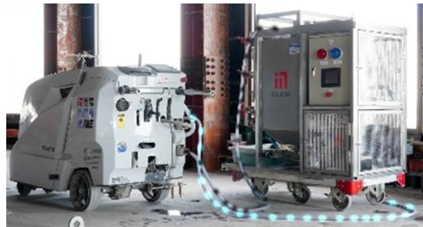
Fig.14. Slurry Water Dewatering Device (Right)
