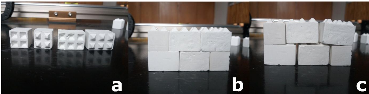
Fig.2 Passive compliance with positioning pegs and holes (tenons and mortises): a) the used elements b) precisely placed elements c) offsets above the manageable limits
