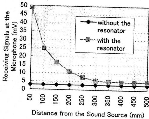
Figure 7. Receiving signals at the microphone of the microrobot in various distances away from the resonator.
