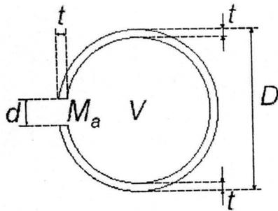
Figure 4: A spherical acoustic resonator.
