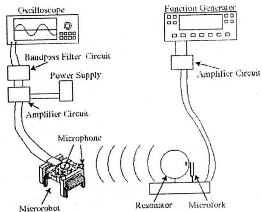
Figure 6: The experiment set-up diagram.
