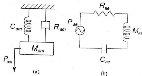
Figure 3: Equivalent circuits of the acoustic resonator: (a) a mechanical circuit, (b) an electrical circuit.
