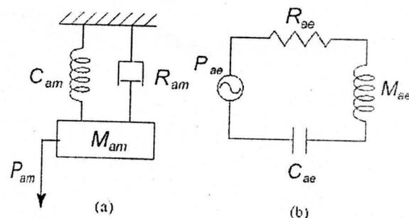
Figure 3: Equivalent circuits of the acoustic resonator: (a) a mechanical circuit, (b) an electrical circuit.
