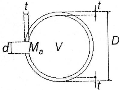
Figure 4: A spherical acoustic resonator.
