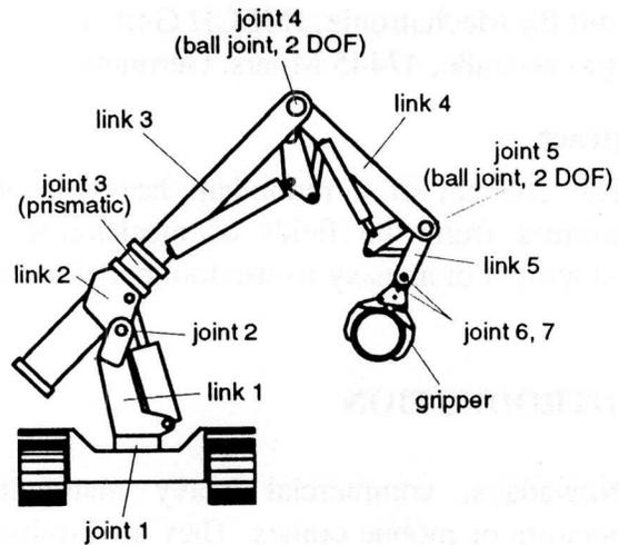
Figure 2: Structure of the redundant manipulator
