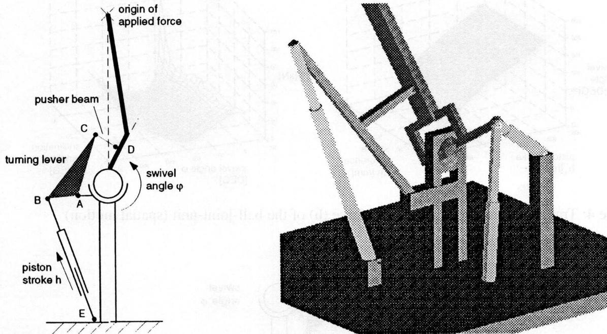
Figure 3: Transmission linkage for a ball joint with three DOF
