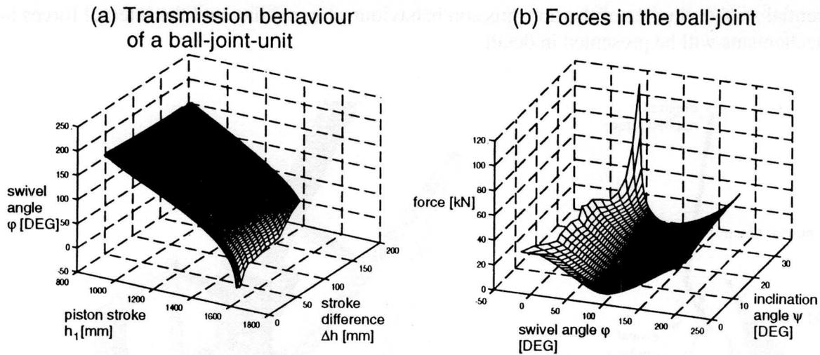
Figure 4: Transmission behaviour (a) and force (b) of the ball-joint-unit (spatial motion)
