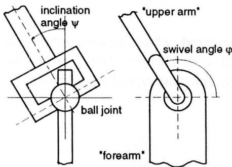
Figure 1: Mobility of a ball joint
