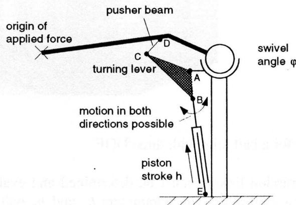
Figure 5: Example for a singular position of the transmission linkage
