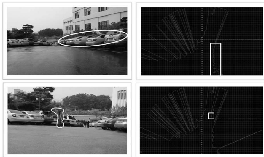
Figure 2 Object Detection by SICK Laser Sensor
