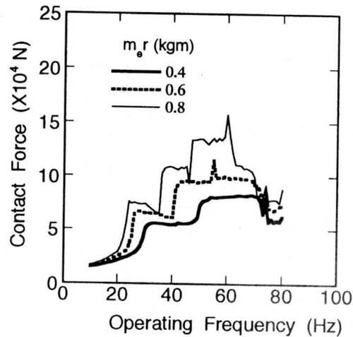
Figure 4 The results for the calculation of the relationship between contact force and frequency with the parameters of eccentric momentum  $m_e r$  ( $m = 1400$  kg,  $k = 12 \times 10^7$  N/m)
