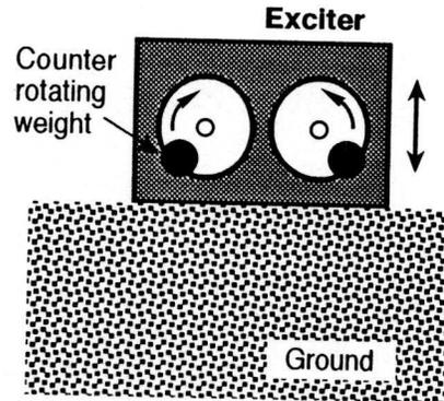
Figure 1 An exciter vibrating on the ground
