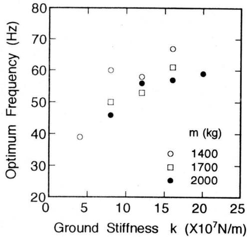
Figure 6 The effects of ground stiffness on the optimum frequency ( $m_{er} = 0.8$  kgm)
