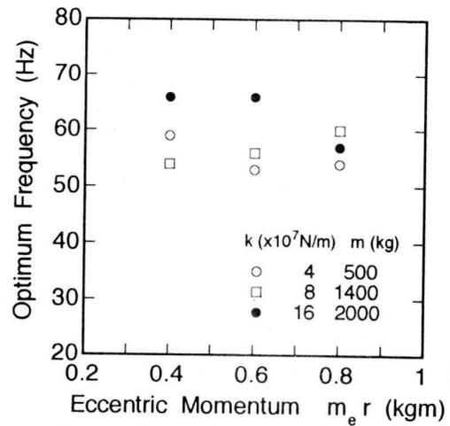
Figure 7 The effects of eccentric momentum on the optimum frequency
