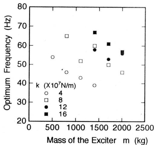
Figure 8 The effects of mass of the exciter on the optimum frequency ( $m_{er} = 0.8$  kgm)
