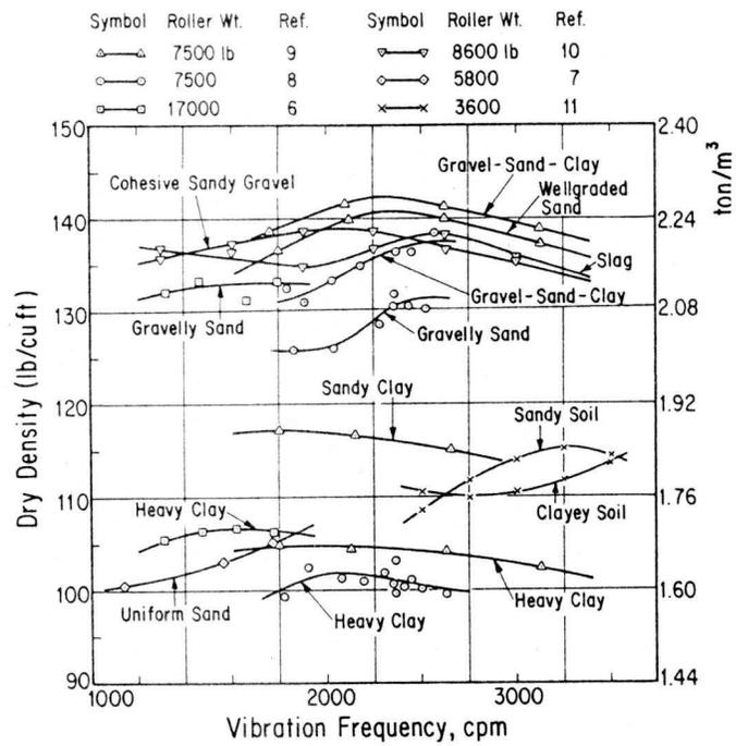
Figure 10 Experimental results of vibratory soil compaction (Selig, E.T., 1977<sup>2</sup>)
