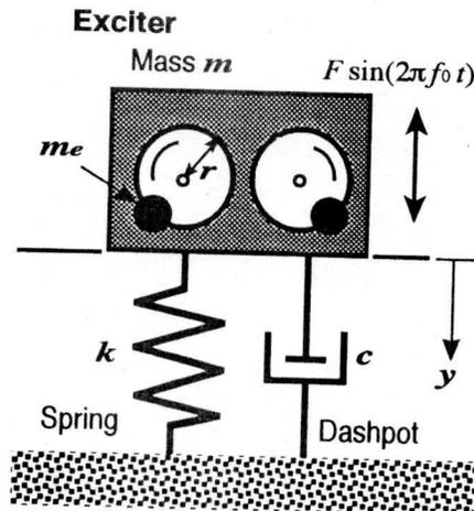
Figure 2 Simulation model for the exciter-ground system
