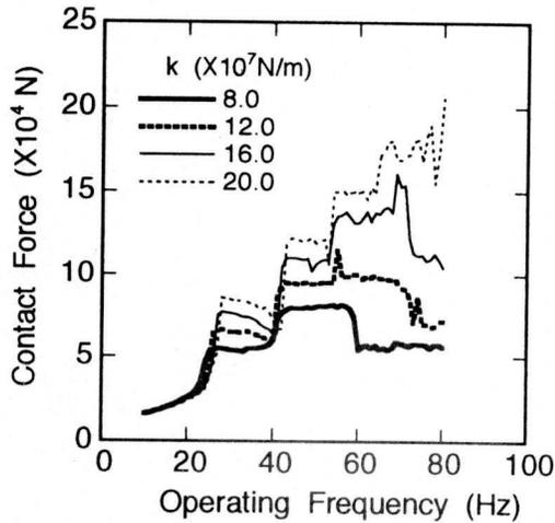
Figure 3 The results for the calculation of the relationship between contact force and frequency with the parameters of ground stiffness  $k$  ( $m = 1400$  kg,  $m_e r = 0.6$  kgm)
