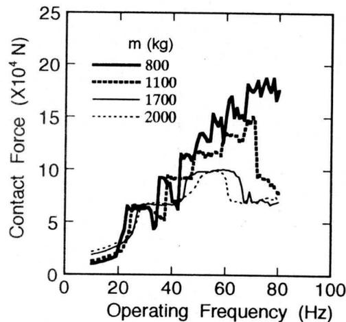
Figure 5 The results for the calculation of the relationship between contact force and frequency with the parameters of mass of the exciter  $m$  ( $m_e r = 0.6$  kgm,  $k = 12 \times 10^7$  N/m)
